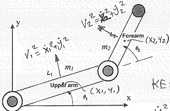
Obtain the equation of motion of this biomechanical model.
