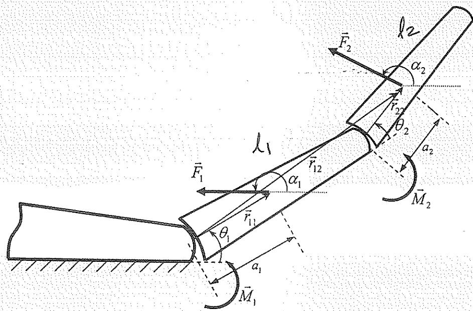
Determine the joint moments  $M_1$  and  $M_2$  in terms of parameters of the physical system shown in the figure. Length of the first and second links are  $l_1$  and  $l_2$ .
