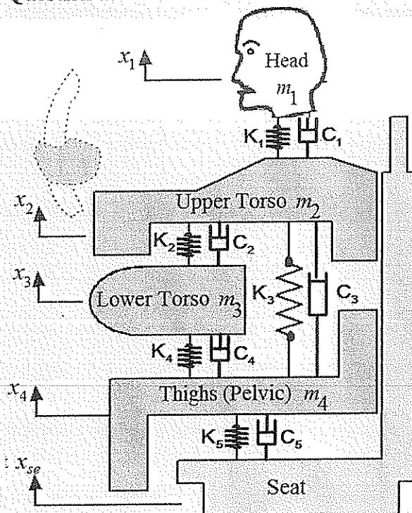
A simplified spring-damper-mass model of the human body created to analyze the effect of vertical vehicle vibrations to human body is shown in the figure. Derive the equation of motion of the corresponding model.
