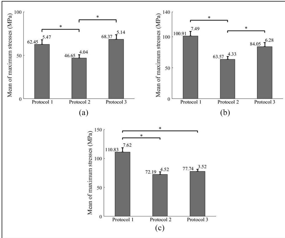
**Figure 6.** Mean ( $\pm$ standard deviation) values of maximum stresses over the mandibles calculated from 10 models under (a) chewing, (b) biting, and (c) impact forces.
