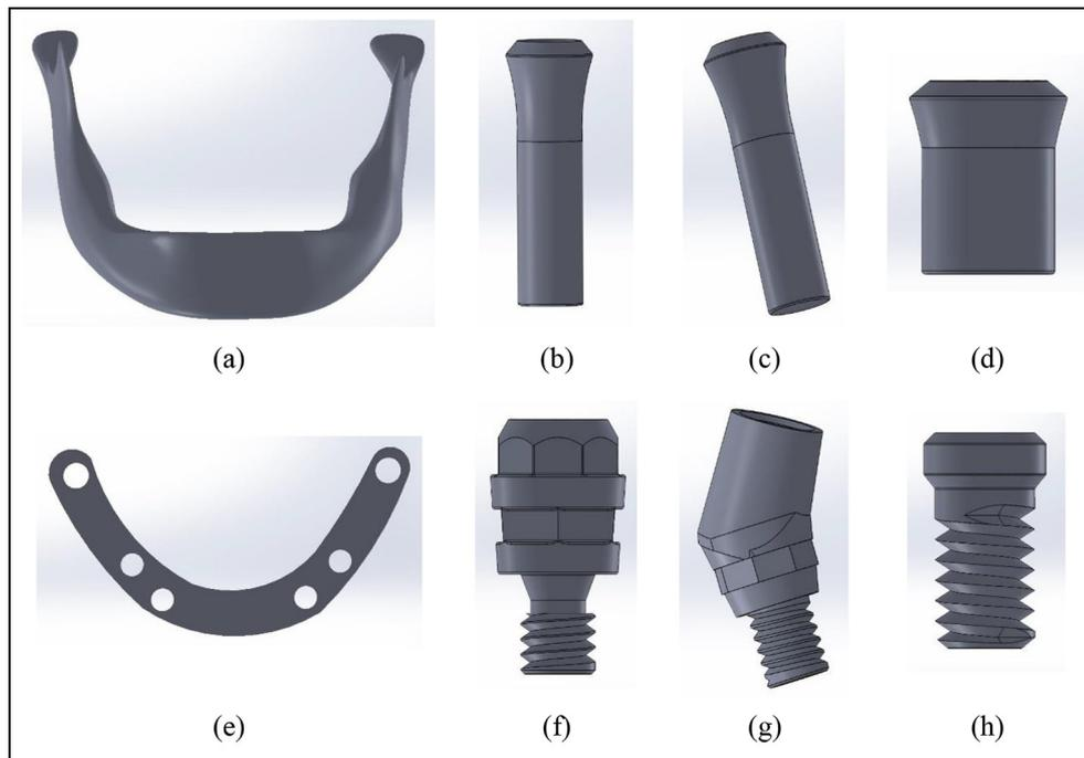
**Figure 1.** The representation of the geometric models: (a) mandible, (b) Straumann<sup>®</sup> regular long implant, (c) Straumann regular long implant tilted with the angle of 30°, (d) Straumann standard plus short implant, (e) prosthetic bar, (f) Straumann cementable abutment, (g) Straumann angled abutment, and (h) Straumann compatible single crowns occlusal screw.
