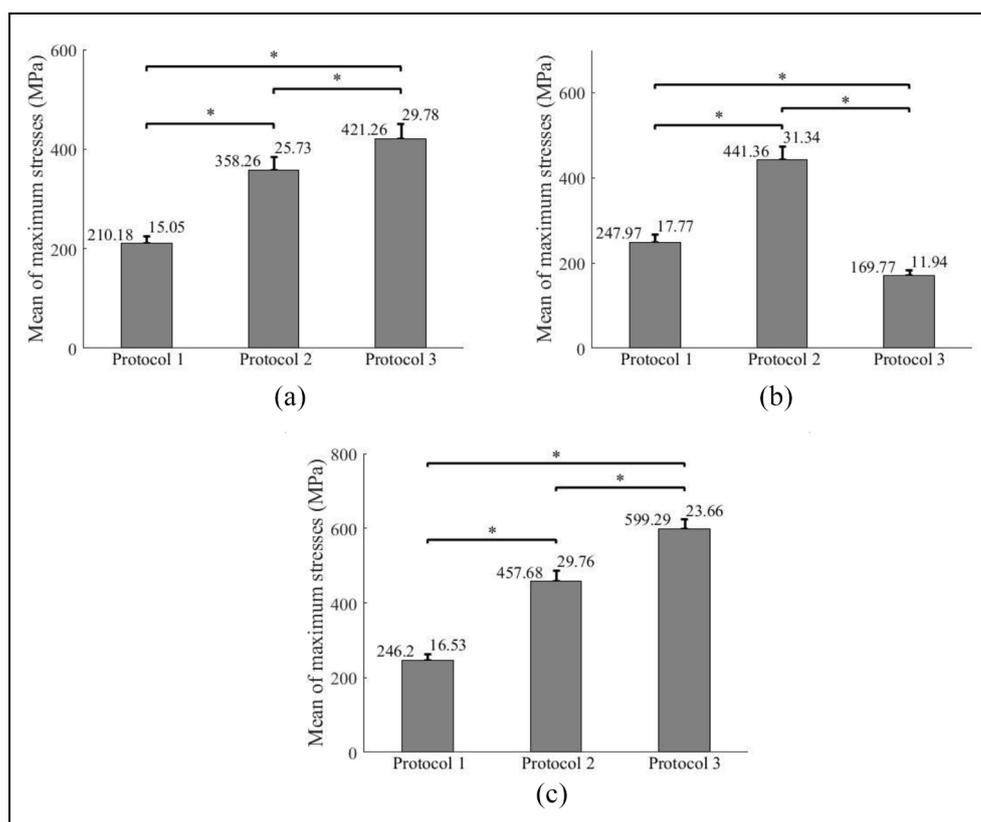
**Figure 8.** Mean ( $\pm$ standard deviation) values of maximum stresses over the dental implants (including both long and short implants together) calculated from 10 models under (a) chewing, (b) biting, and (c) impact forces.
