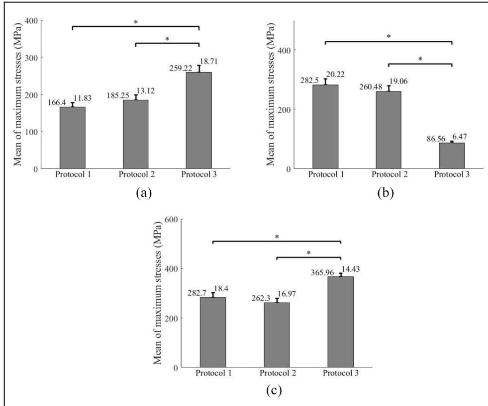
**Figure 9.** Mean ( $\pm$ standard deviation) values of maximum stresses over the abutments calculated from 10 models under (a) chewing, (b) biting, and (c) impact forces.
