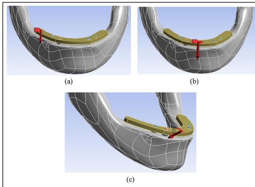
**Figure 4.** Loading conditions: (a) chewing force, (b) biting force, and (c) impact force. The magnitude of all forces is 62.8 N.
