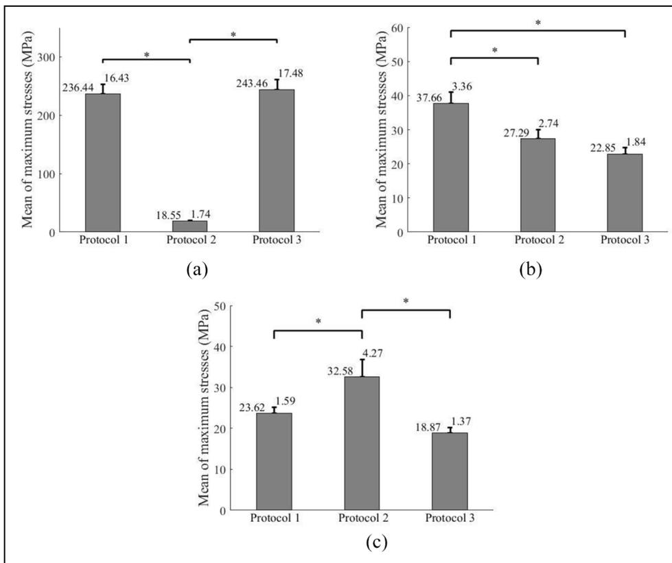
**Figure 7.** Mean ( $\pm$ standard deviation) values of maximum stresses over the prosthetic bars calculated from 10 models under (a) chewing, (b) biting, and (c) impact forces.
