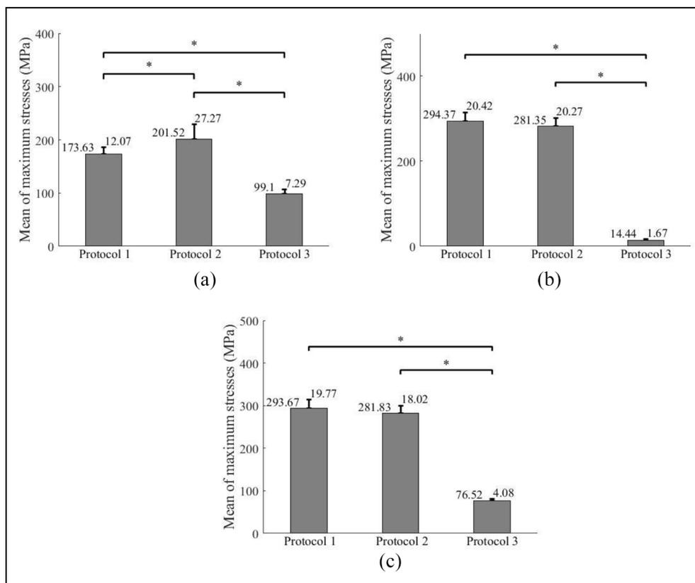
**Figure 10.** Mean ( $\pm$ standard deviation) values of maximum stresses over the screws calculated from 10 models under (a) chewing, (b) biting, and (c) impact forces.
