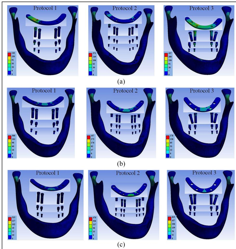
**Figure 5.** Representative von Mises stress distributions over the mandible, prosthetic bar, dental implant, abutment, and screw under (a) chewing force, (b) biting force, and (c) impact force (all stress values are in MPa).
